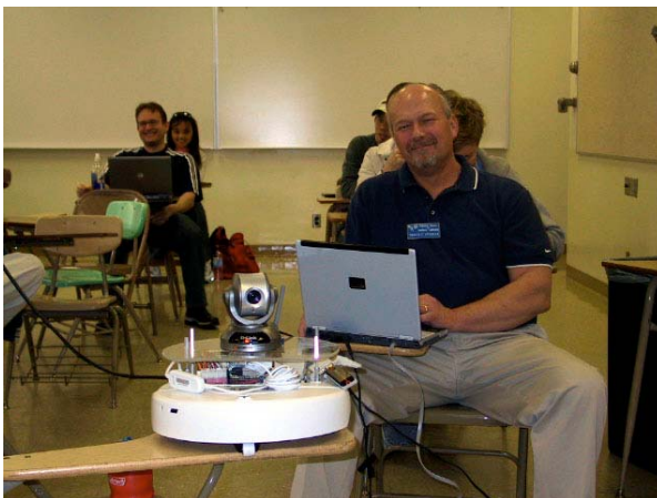
Terrence Everett demo'd his iCreate robot with an ITX processor installed. He also is using RoboRealm software with this robot. He's also installed his wireless Dlink pan and tilt camera and demonstrated its abilities to pan/tilt, zoom, autofocus etc.
